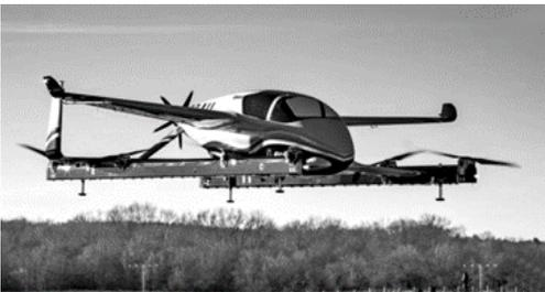
Boeing successfully completed the first test flight of its autonomous passenger air vehicle (PAV) prototype in Manassas, Virginia. Boeing NeXt, which leads the company's urban air mobility efforts, utilized Boeing subsidiary Aurora Flight Sciences to design and develop the electric vertical takeoff and landing (eVTOL) aircraft and will continue testing to advance the safety and reliability of on-demand autonomous air transportation.
