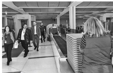
In an effort to expedite the screening process for our customers without sacrificing security, we recently partnered with the TSA to install a new computed tomography (CT) scanner in ORD's Terminal 1. This technology allows TSA agents to view a three-dimensional image of a passenger's carry-on bag and focus in on specific items, such as liquids or laptop computers, that require additional attention.
