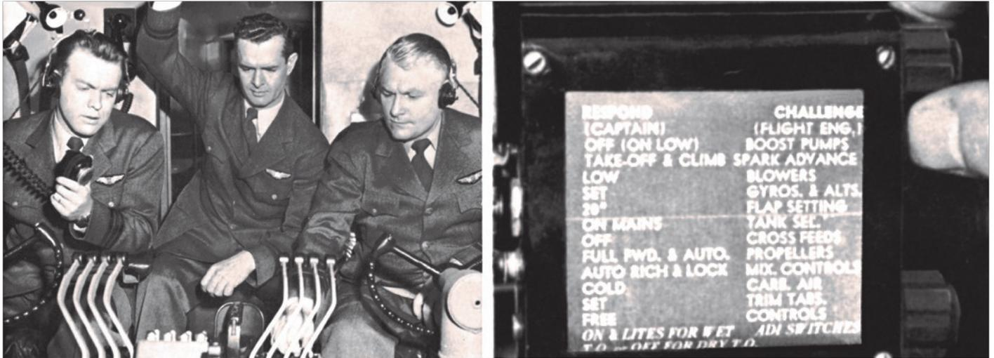
A “Challenge and Response” check was the last inspection of the DC-6’s instruments and controls after the engines were run-up to cruise power prior to take-off. The scroll shows a portion of the “oral challenges” made by the Flight Engineer and “responded to” by the Captain as he made the required checks. After
