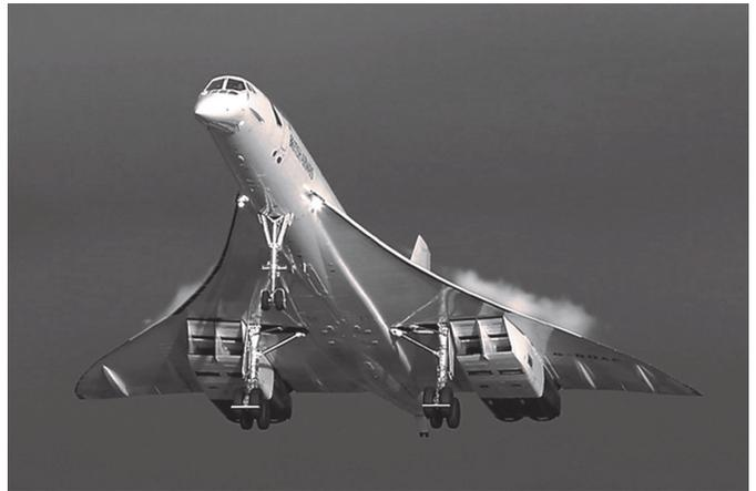
Dry thrust: 32,000 lbf each. Thrust with afterburner: 38,050 lbf each. (*Not really a whole lot! B*)
