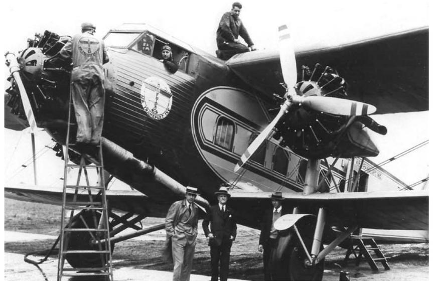
The pilot and co-pilot sat in a separate forward cabin and were kept informed of changing weather conditions by two-way radio. The plane was soon redesigned to carry 18 passengers and designated the "Model 80A" (photo). The "80A" was powered with three 525 hp Pratt & Whitney "Hornet" engines with a cruising speed of 125 mph and a range of 460 miles. The gross weight was 17,500 pounds.
